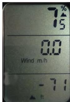
To set the correct elevation, while in the Slope/Wind/Elevation screen, press-hold the center button for a few seconds. The current elevation will be updated to the reference elevation memorized earlier in the Set Alt step.
