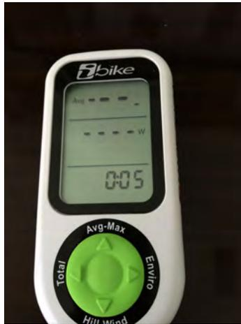
**NOTE:** IN THE TOP WINDOW THE LEAST SIGNIFICANT DIGIT OF THE AVERAGE WATTS NUMBER WILL BE SUBSCRIPTED. FOR EXAMPLE, AN AVERAGE WATTAGE OF 198W WILL SHOW IN THE TOP WINDOW AS 19<sub>8</sub>
