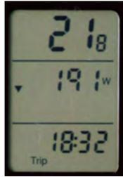
This screen shows that this rider has 18 minutes, 32 seconds remaining on the test (bottom window), and that, up to this point of the test, the rider has sustained an average of 218W (top window). The middle screen shows the watts output at the instant of the photo: 191W. So, the rider's wattage output AT THAT INSTANT is below the average. The down arrow to the left of the reading 191W indicates that the instantaneous wattage output is below the average watts output.
