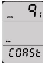
17. Once you get to a speed of about 8 mph, the words "DONE COAST" will flash for a few seconds, then the screen "CALC COAST" (calculating coast) will appear, then main coast down screen will appear, indicating that the measurement is complete.
