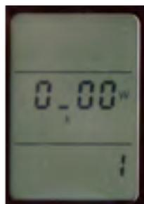
Your watts-per-kilogram (W/KG) number will be shown in the center window: x\_yz, where x,y and z are numbers, and the underscore indicates a decimal point. For example, 3\_54 indicates a watts/kg result of 3.54. The bottom window shows your fitness level associated with your W/KG test result.
