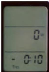
The instant you start pedaling the bottom window clock will start counting down to zero. *When the clock reaches 0:00 the test will begin and the timer will reset to 20 minutes, zero seconds, and count down towards zero.*
