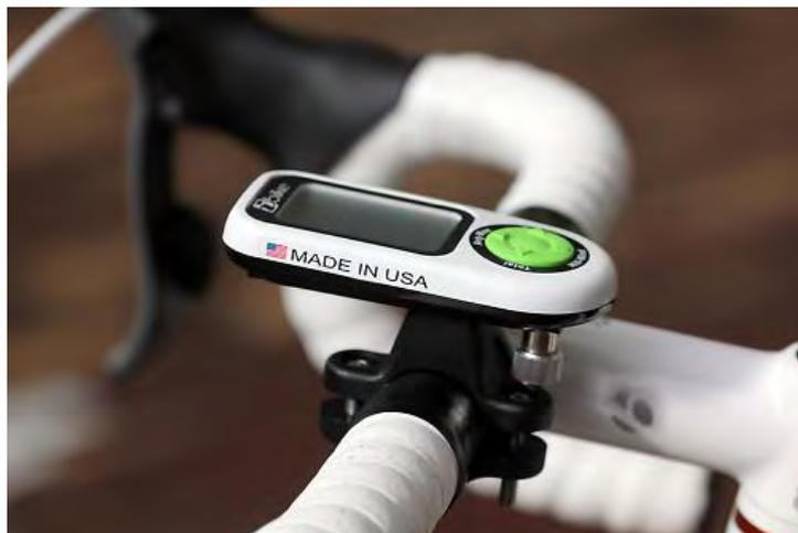
The system comprises a wireless speed/cadence sensor (20g) that you mount on your chainstay and a head unit (72g) that fits on a mount (44g)
