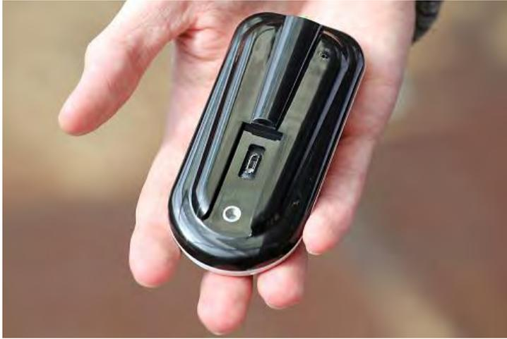
Once fitted, you have to perform a 10 minute 'calibration ride' which simply involves riding along an open road for five minutes, turning around and riding back. This calibrates the Newton's wind and tilt sensors.
