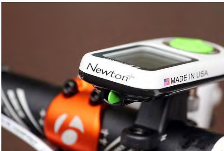
The Newton takes the air pressure, accelerometer and speed measurements to calculate the total force working against you. The total opposing force multiplied by your speed gives your power.
